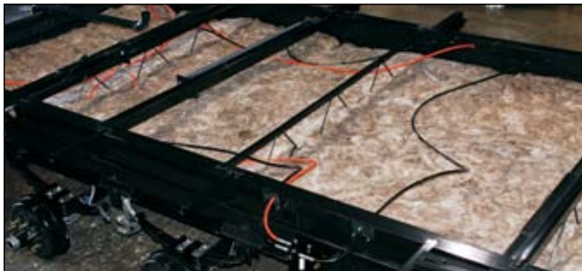
All aluminum sills and wall studs are mechanically joined and the aluminum sill tubing is fully reinforced internally with wood, providing greater strength and stability when it is "bolted-through", never screwed, to the sub-floor structure and the steel frame below.
