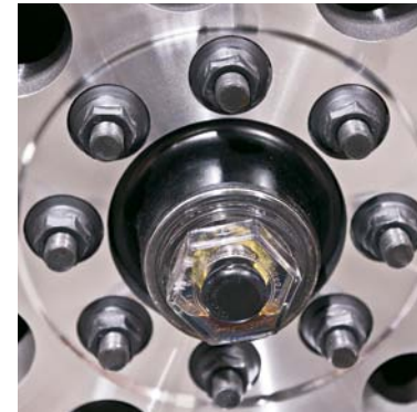
Commercial oil bath hubs surrounded by 8 large 5/8" stud bolts and standard automotive disc brakes round out the safety features of every DRV unit.
